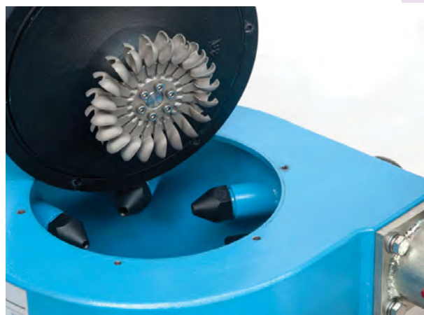
Detail of Pelton turbine and distributors
