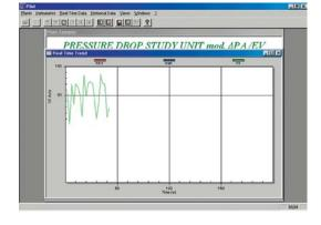
There is no need of inserting any card in the PC to use this software; it is sufficient to connect the plant with the serial port (COM1 or COM2) of the P.C. via the serial cable of the equipment.
