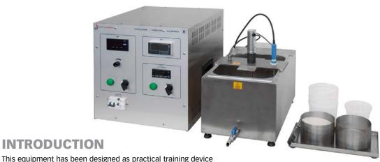
This equipment has been designed as practical training device for cheese making technique; it consists of a control unit and of a cheese vat.
